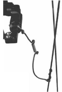
14. TM style rests should have the spring tension set so that the rest remains in the full upright position before the bow is drawn back.
