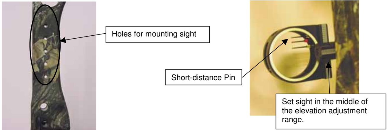
18. Secure the bow in a bow vise in a level position. Adjust the bow so that it is level. Place a leveling device on a flat surface of the sight mounting bracket. With the bubble in the leveling device centered, adjust the sight so that the bubble in the sight is centered.
