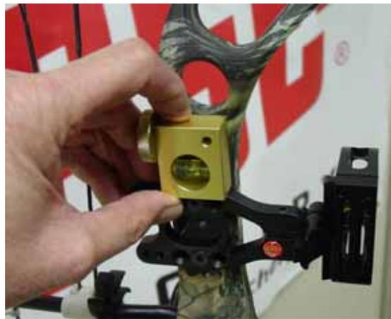
19. Adjust the third axis of the sight. Check the third axis leveling by tilting the bow forward. The levels on the sight and the riser should still be centered. Then tilt the bow to the rear and make the same check.
