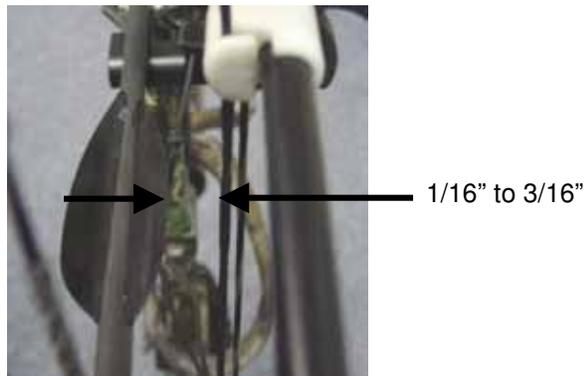
16. Set peep height and tie in the peep. Tie in the peep with serving material. Slide the peep either up or down so that it is approximately even with the eye when the bow is in the fully drawn position.
